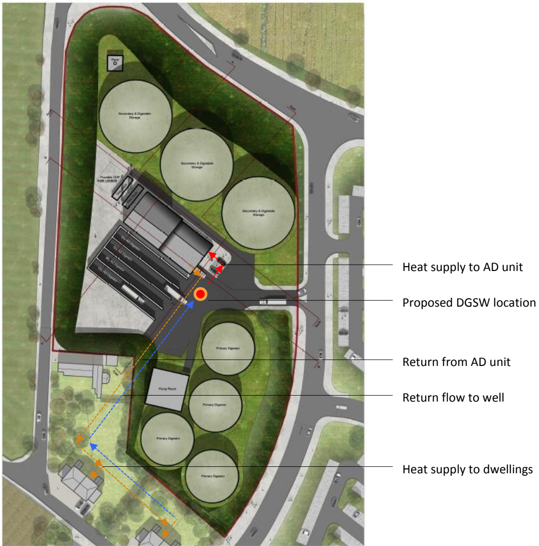
Figure 11 Proposed location of the single well and associated pipework to supply heat to the AD unit and residential dwellings
