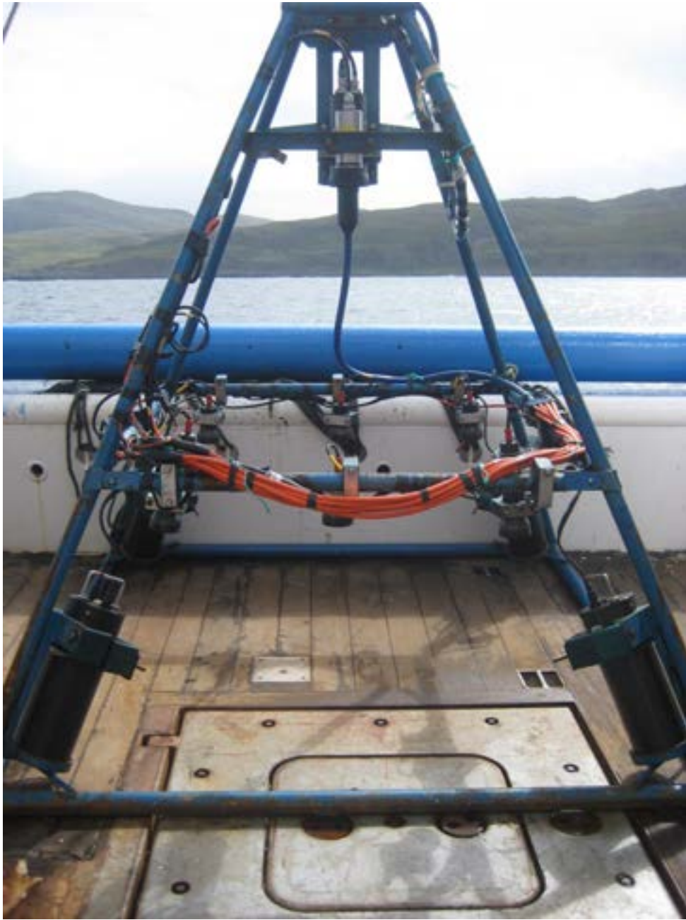
The camera drop frame prior to its deployment from the aft deck of FRV Alba na Mara .
