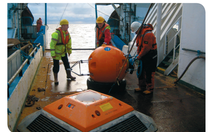
PROFILING CURRENT METERS READY FOR DEPLOYMENT IN THE FAROE SHETLAND CHANNEL.
