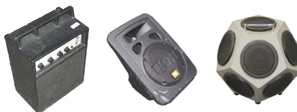
Figure 3 Typical loudspeaker used during airborne sound insulation tests
