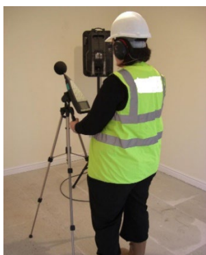
Figure 1 Sound test being carried out
