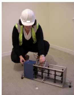
Figure 4 Impact sound test being carried out
