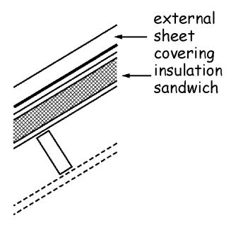
Note Roof type (D) is not suitable for sheet metal coverings that require joints to allow for thermal movement. See also sub-clause f of clause 3.10.1.
