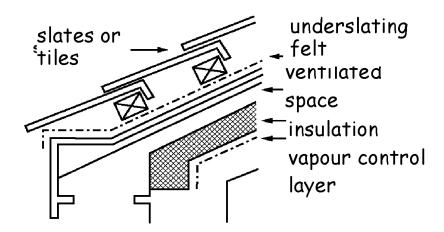
Roof type C (slate or tiles - insulation on decking) - pitched roof structure as (A) above with a decking of low permeability insulation fitted to and between the roof framing. External weatherproof covering of slates or tiles, with tiling battens and counter battens (located over roof framing), and a breather membrane laid on the insulation decking; with a sloping ceiling.
