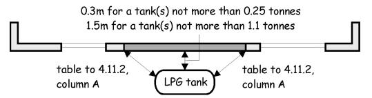
Motor vehicles under the control of a site occupier should be parked at least 6m from LPG tanks or the separation distance in column (A) of the table to this clause, whichever is the smaller. This does not apply to the loading/unloading of vehicles. Motor vehicles not under site control (e.g. those belonging to members of the public) should be parked no closer than the separation distance in column (A) of the table to this clause.
