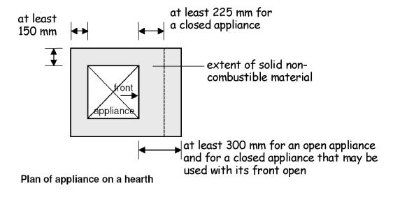
The 150mm does not apply where the appliance is located in a fireplace recess, nor does it apply where the back or sides of the hearth either abut or are carried into a solid, non-combustible wall complying with clause 3.19.8.
