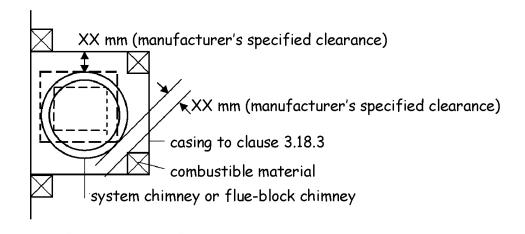
BS EN 1806: 2000 relates to clay flue-block chimneys but does not give a value for distances to combustible materials. These types of chimneys therefore should be regarded as a custom built chimneys and the minimum values in this clause 3.19.1 or clause 3.19.2 should be used and declared.
