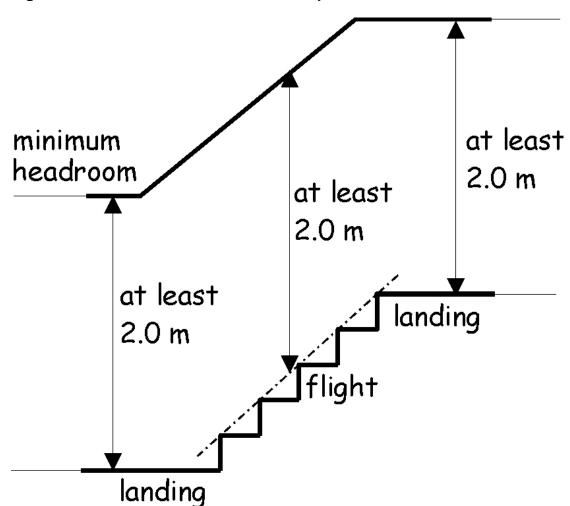
Figure 4.11 Headroom on stairs and ramps
