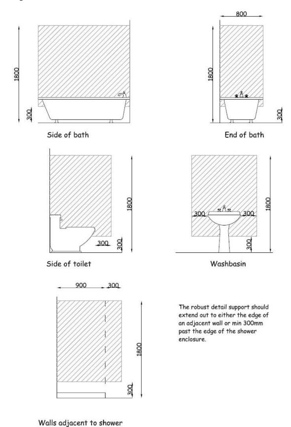
Examples of robust wall construction include masonry walling and suitably reinforced timber and metal stud partitioning. The following sketches indicate how timber or metal stud partitioning may be reinforced in preparation for the future installation of grab rails.
