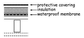
Roof type E (troughed metal decking - warm roof) - flat roof structure of timber or metal framed construction with a troughed metal decking; with or without a ceiling or soffit. External weatherproof covering and insulation and vapour control layer as (A) above. [Note 1]
