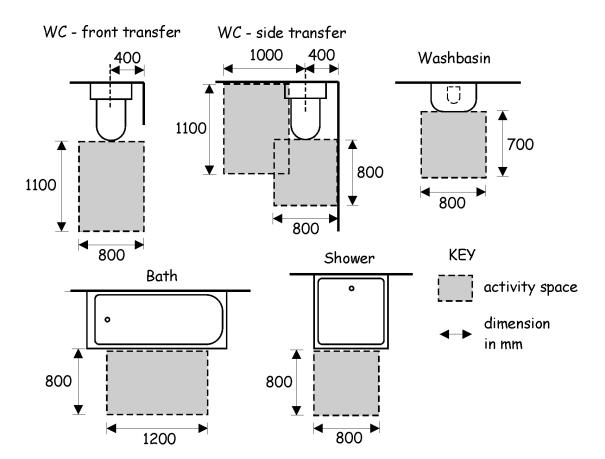
Figure 3.31 Activity spaces for accessible sanitary facilities
