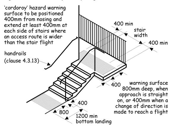
Figure 4.8 Use of corduroy tactile paving
