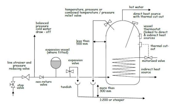
Figure 4.12 Unvented hot water storage system – indirect example
