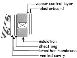
Wall type C (sheet or panel cladding with/ without ventilated cavity) - framed wall of timber or metal studs and dwangs. Sheet or panel cladding material of fibre cement, plastic, metal, GRP or GRC. Insulation applied either to the internal face of the framing with permanent ventilation behind any impervious cladding, or as an infill to the framing; in either case the wall lined internally with a vapour control layer and a
