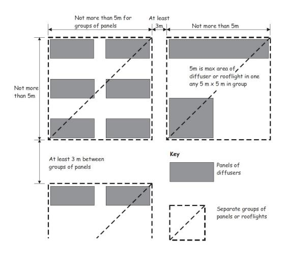
Figure 2.2 Layout restrictions on small TP(b)rooflights and light fittings with diffusers
