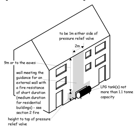
Figure 4.14 Small LPG tank close to a building
