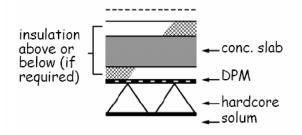
Damp-proof membrane above or below the slab or as a sandwich; jointed and sealed to the damp proof course or dampproof structure in walls, columns and other adjacent elements in accordance with the relevant clauses in section 3 of CP 102: 1973.
