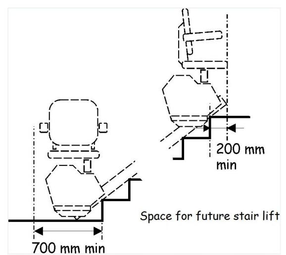
Figure 4.5 Future provision for unassisted access
