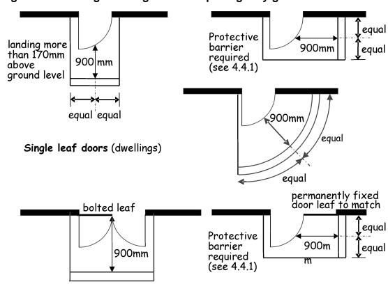
Figure 4.9 Landings serving outward-opening fully glazed doors
