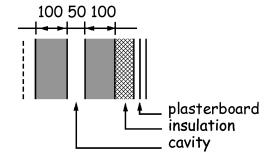
Wall type B (cavity wall with cavity fill insulation) - Cavity wall as (A) above. Wall rendered or unrendered externally. Insulation applied as a cavity fill. Wall with or without an internal surface finish of plaster or plasterboard. This construction is only recommended for sheltered conditions.
