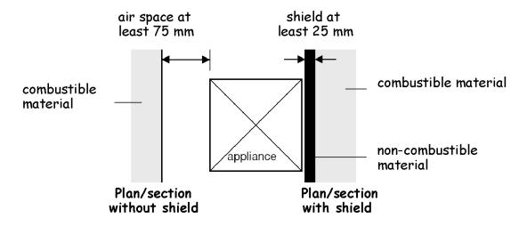
A gas-fired appliance with a CE marking and installed in accordance with the manufacturer's written instructions may not require this separation.
