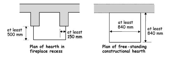
Not only should a solid fuel appliance sit on a hearth, but the appliance itself should also be located on the hearth such that protection will be offered from the risk of ignition of the floor by direct radiation, conduction or falling embers. The solid fuel appliance should be located on a hearth in accordance with the following diagram:
