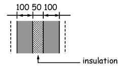
Wall type C (cavity wall with partial fill insulation) - Cavity wall as (A) above. Wall rendered or unrendered externally. Insulation applied to either leaf as a partial cavity fill so as to preserve a residual space of 50mm wide. Wall with or without an internal surface finish of plaster or plasterboard.
