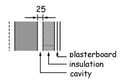
Wall type B (solid wall with external insulation)- Solid wall as (A) above. Insulation applied to the external surface of the wall; protected externally either by cladding (of sheets, tiles or boarding) with permanent ventilation, or by rendering. Wall with or without an internal surface finish of plaster or plasterboard.
