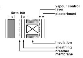
Wall type B (weatherboarding, tile or slate Figure 3.17 Wall type B
