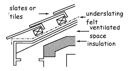
**Roof type B (slate or tiles - insulation on a sloping ceiling)** - pitched roof structure as (A) above. External weatherproof covering as (A).
