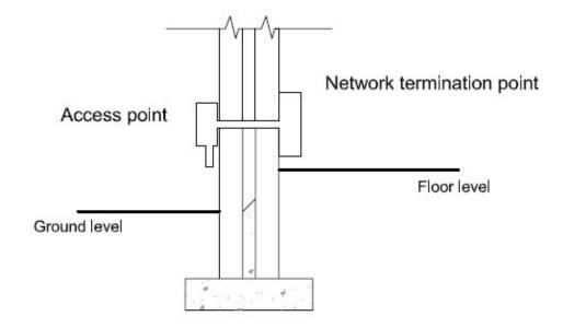
In flats and maisonettes the in-building physical infrastructure should be taken to an individual network termination point within each flat or maisonette. Such infrastructure may consist of a single duct from a main access point outside the building, leading to a common access point within the building, which is usually located in a communal service riser. The infrastructure from the common access point to the individual termination points may be either:
