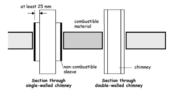
There should also be a separation distance where the metal chimney runs in close proximity to combustible material. The separation distance should be 25mm from the outer surface of a single-walled chimney to combustible material. The 25mm should be measured from the surface of the inner wall of a double-walled chimney. There is no need for a separation distance if the flue gases are not likely to exceed 100°C.
