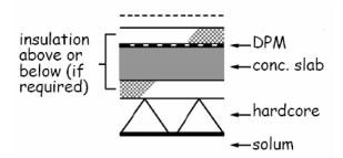
Concrete slab 100mm thick with insulation, if any, laid above or below the slab; with or without a screed or floor finish.
