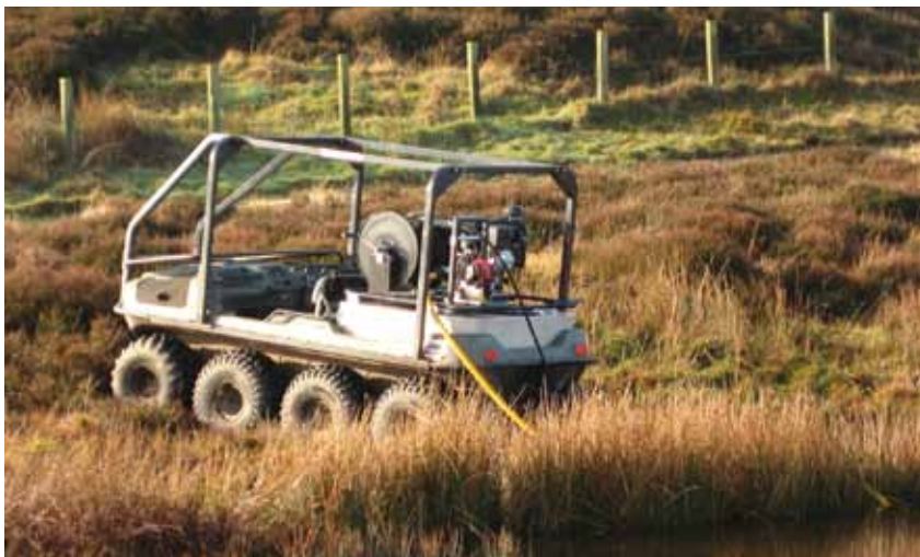
◀ Photo 8A.3 An Argo-cat All-Terrain Vehicle (ATV) available to Northumberland fire group partners
