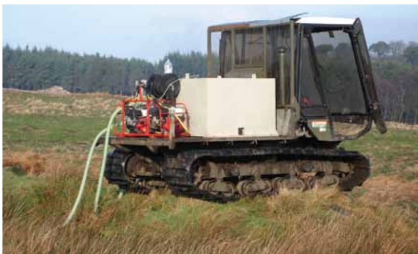
Photo 8A.7 A soft track vehicle equipped with a fire fogging system
