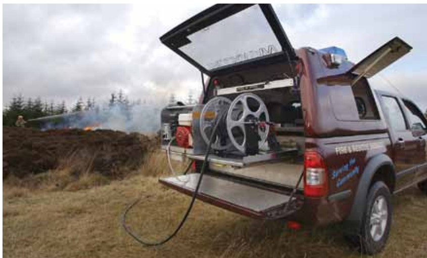
Photo B8.1 A photograph of a wildfire vehicle equipped with a fogging unit which can provide water support to hand crews
