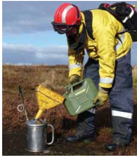
◀ Photo B10.9 Correct re-filling of a drip torch – full PPE, away from ignition sources and preventing spillages
