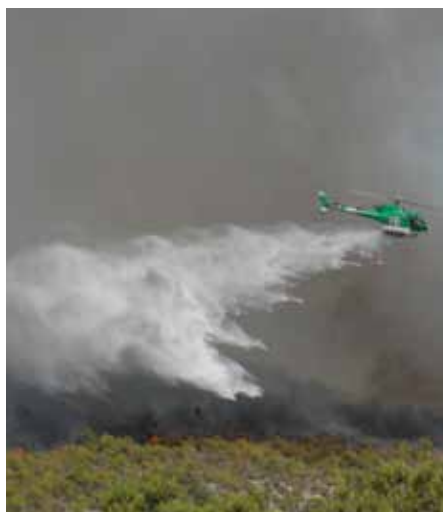
◀ Photo B9.12 A wide drop made from fixed water tanks
