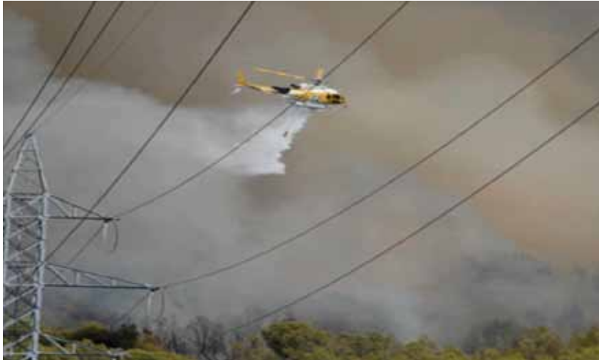
< Photo B9.3 Overhead powerlines are a significant risk to aircraft
