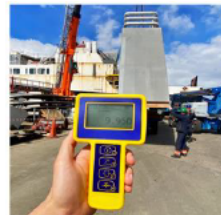
Proof of load test carried out on largest testing 470 Ton Site.
