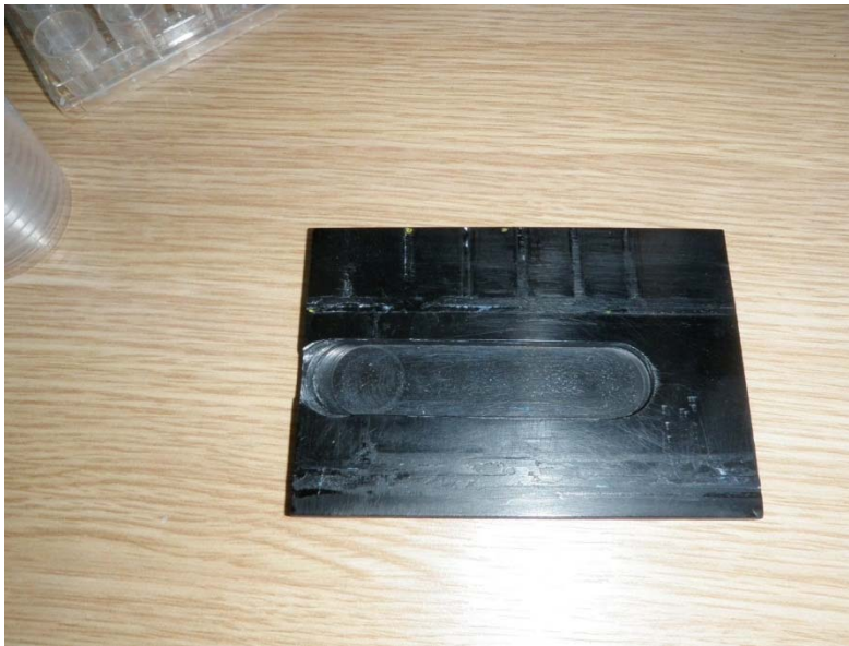
Figure 2. Bespoke plastic tray used for reading anglerfish and megrim otoliths.
